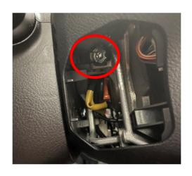
**Step 4:**Pull airbag up and place as shown, do not disconnect wiring. It may be necessary to slightly pull the torx screws to fully release airbag, do not
